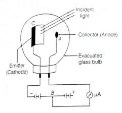
Thus, the photoelectric current sets up in the photoelectric cell corresponding to incident light, it provides the information about the objects as has been seen by our eye in the presence of light.
